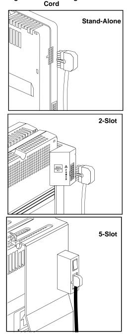
Figure 2-16. Attaching the Power
