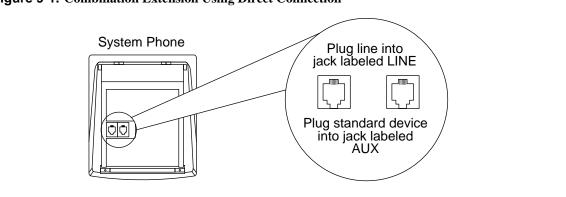
Figure 9-1. Combination Extension Using Direct Connection
