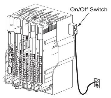
Figure 10-1. On/Off Switch on a 5-Slot Carrier
