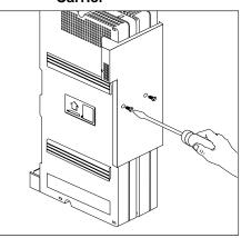
Insert the 3-1/2 inch #8 screw into the bottom of the modules (see Figure ). Tighten it until the mounting tracks of the PARTNER ACS processor module are flush against the wall. Do not overtighten or the module will warp. Then go to the next procedure, "Labeling Jacks" on page 2-9.
