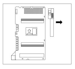
6. Slide the top module to the left to disengage its interlocking mounting tracks from the processor module.
