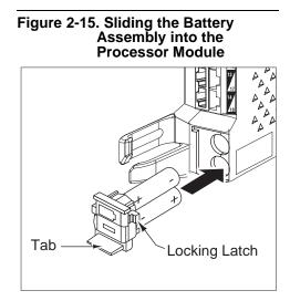
6. Pressing lightly on the battery icon on the front of the battery assembly, slide the locking latch downward to secure the assembly in place. The "plus" icon and the battery icon should now be visible on the front of the battery assembly (see Figure 2-13).
