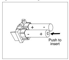
5. With the locking latch in the unlocked position (battery icon and "minus" icon visible), slide the battery assembly into the processor module along the battery guides on the inside of the battery compartment (see Figure 2-15). Push the battery assembly in far enough that the edges of the assembly slip behind the plastic housing of the processor module.
