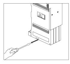
4. Remove the screws that attach the carrier to the modules (see Figure 10-6).
