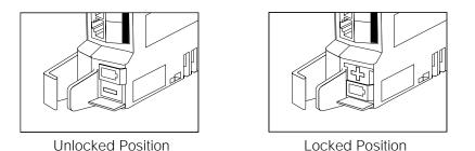
Figure 6-5. Battery Assembly in Unlocked and Locked Position
