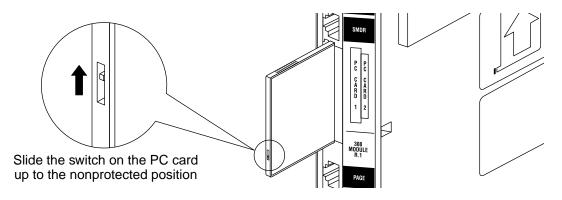
Figure 6-6. Write-Protect Tab on a Backup/Restore PC Card
