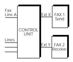
Figure 4-10. Send and Receive Fax Machines
