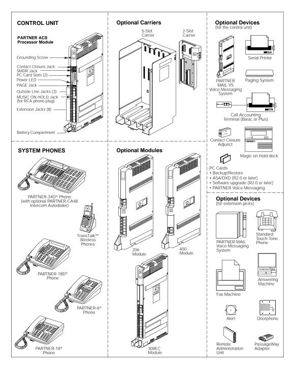
Figure 1-1. Sample System Components
