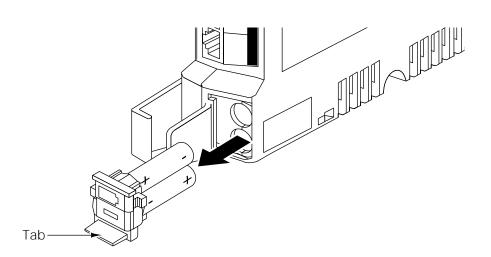
Figure 6-2. Removing the Battery Assembly
