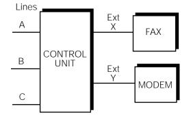
Figure 4-13. Night Service with Fax Machine and Modem
