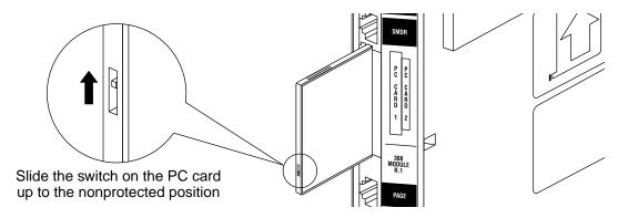
Figure 6-7. Write-Protect Tab on a Backup/Restore PC Card
