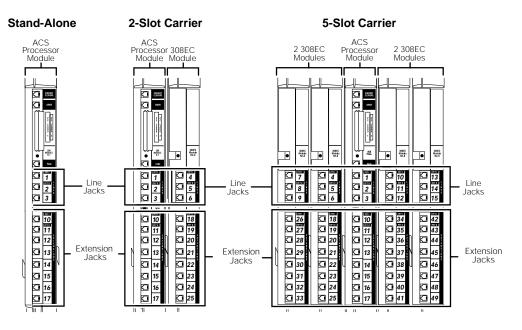
Figure 2-2. Standalone, 2-Slot, and 5-Slot Systems Configured for Maximum Extensions (8, 16, or 40)
