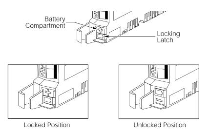
Figure 6-1. Battery Compartment, PARTNER Advanced Communications System Processor Module
