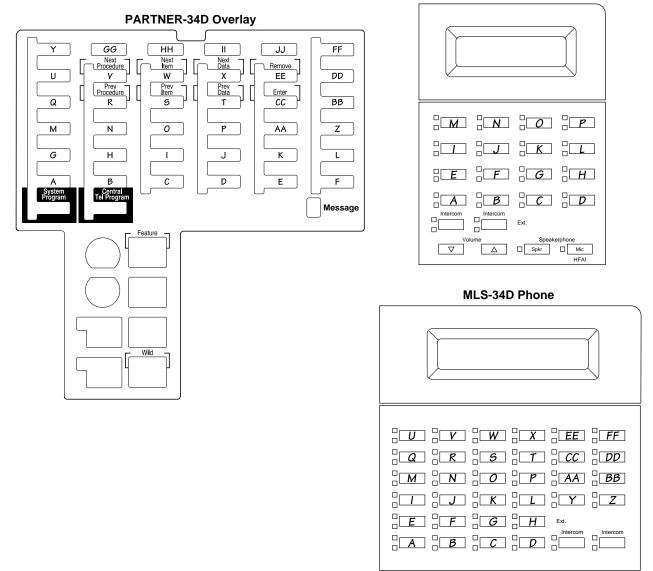
Figure D-2. Programming from an MLS-34D Phone
